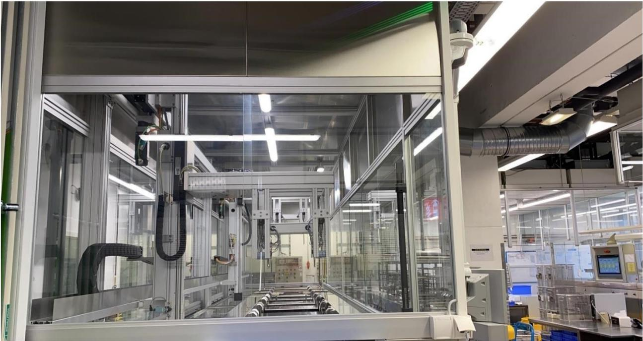
The transport racks of the two transfer units have different grippers to pick up the various cleaning containers provided by the customer and carry out program-specific movements of the containers in the treatment stations.
