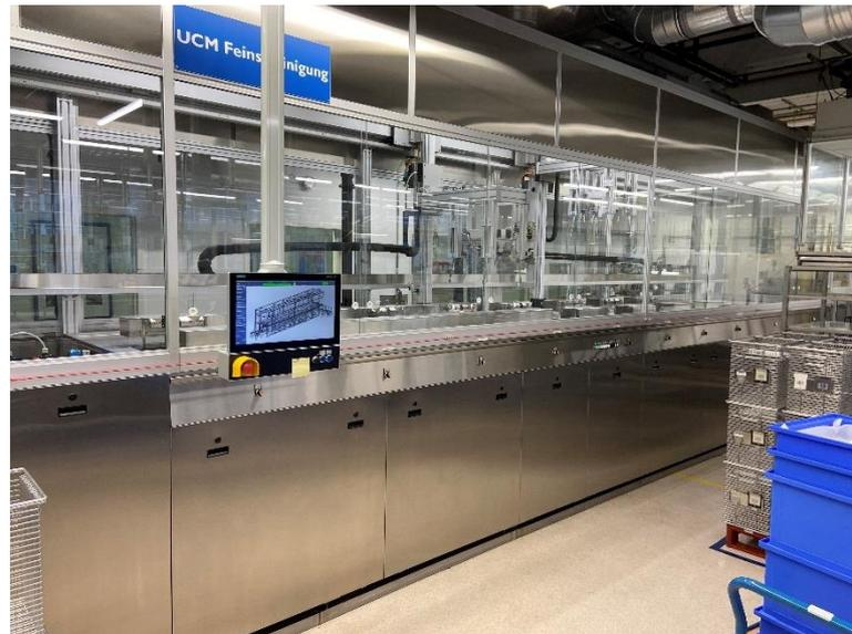
The ultrasonic fine cleaning system, equipped with twelve treatment stations, ensures that the cleanliness specifications of two or less particles of 5 µm or one or less particle of 10 µm are reliably met when X-ray tube parts receive their final clean.
