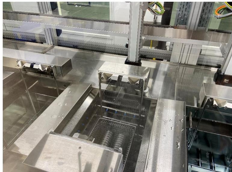
The integrated spray rinse with deionized water removes even very fine dust particles still sticking to the surface after cleaning and the first immersion rinse.
