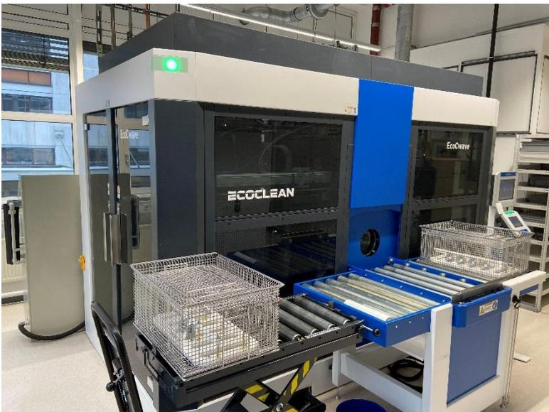
The components of spiral groove bearings are to be cleaned in a standard machine. Cleaning tests before the investment showed that only the EcoCwave can achieve the required results.
